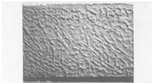
FIG. 8. Surface roughening of the 20Mo55Fe25Ni alloy during oxidation at 910°C. Top, surface roughening as a function of time ( 1\times before reduction for publication); bottom, surface after 224 min. ( 5\times before reduction for publication.)
