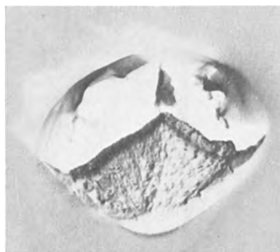
FIG. 7. Crystalline area with 2 segments. 15,000 \times
