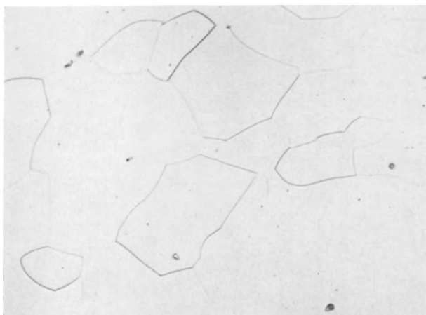
FIG. 5. Recrystallized grain structure of iodide-chromium sheet fabricated at 700°C and annealed 1 hr at 1000°C. Oxygen content of 0.0074%; note the rounded, gray, oxide inclusions; electrolytic etch in 10% oxalic acid. 500X.
