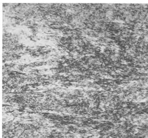
FIG. 8. Cold rolled and annealed structure of electrolytic titanium, 90% reduction, top view.
