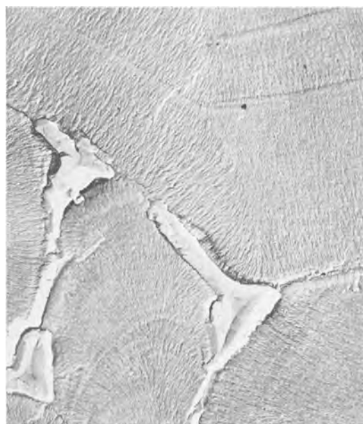
FIG. 9. Intersections of crystalline areas on a specimen almost completely crystallized. 5000 \times .
