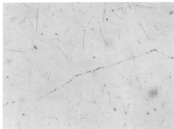
FIG. 12. As-cast structure of chromium containing 0.124% nitrogen and 0.059% oxygen. Large, light-colored Widmanstätten rods and grain boundary precipitate of nitrogen-rich phase plus gray-colored oxide inclusions; electrolytic etch in 10% oxalic acid. 500X.
