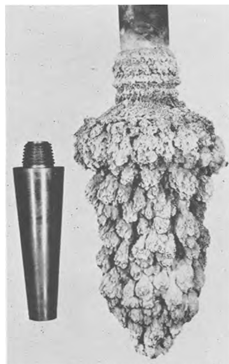
FIG. 6. Zirconium cathode deposit compared with typical mild steel cathode.
