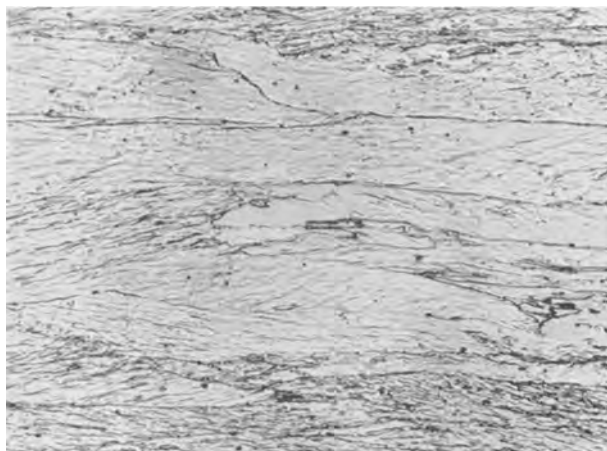
FIG. 4. Longitudinal fibered grain structure of iodide-chromium sheet rolled at 700°C. Oxygen content of 0.0093%; electrolytic etch in 10% oxalic acid. 250X.
