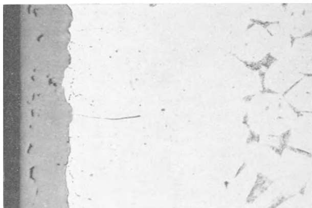
FIG. 7. Zirconium-1.5 wt % tin alloy reacted with oxygen at 825°C for 180 min. Surface layer is a gray-black film about 0.0025 cm thick. Aqua regia-HF etch. 500X before reduction for publication.
