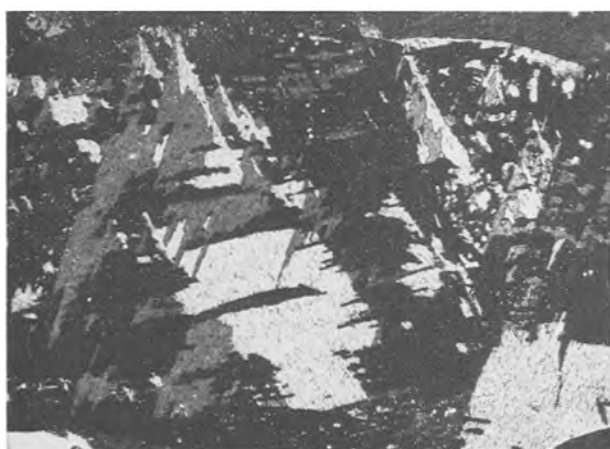
FIG. 6. Twice arc melted electrolytic titanium as-cast structure showing large coarse grains of high purity metal.
