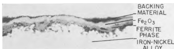
FIG. 2. Oxide film on iron-nickel alloy prepared by sand blasting. Oxidized for 60 min at 700°C. 2000× before reduction for publication.
