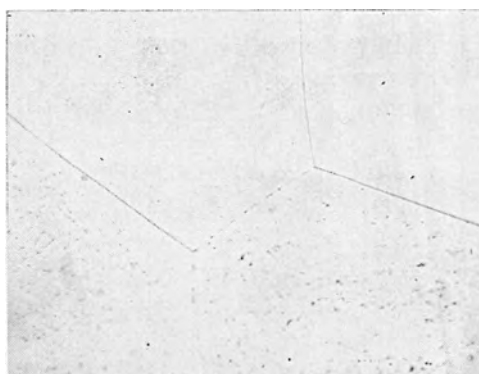
FIG. 6. Microstructure of arc-melted calcium-reduced molybdenum. Etchant, \text{NH}_4\text{OH}\text{-H}_2\text{O}_2 . 500 \times before reduction for publication.
