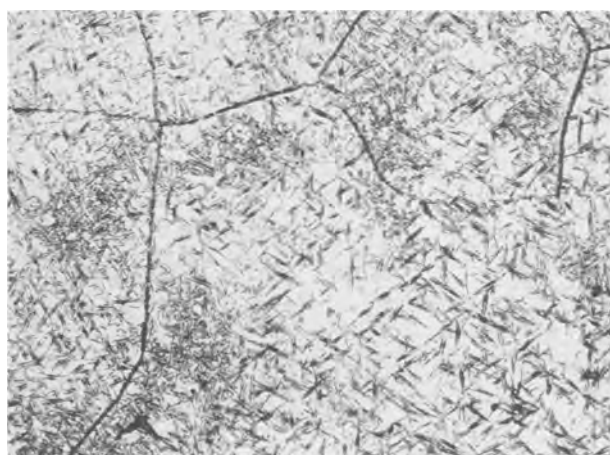
FIG. 7. Arc melted as-cast titanium surface, Widmanstatten structure. Electrolytically polished and etched.
