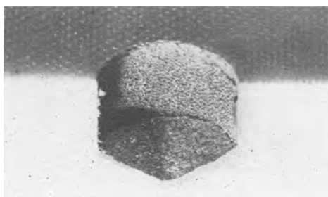
FIG. 4. Cross-sectional view of \frac{1}{2} in. diameter tapered cavity drilled in glass silicone laminate.
