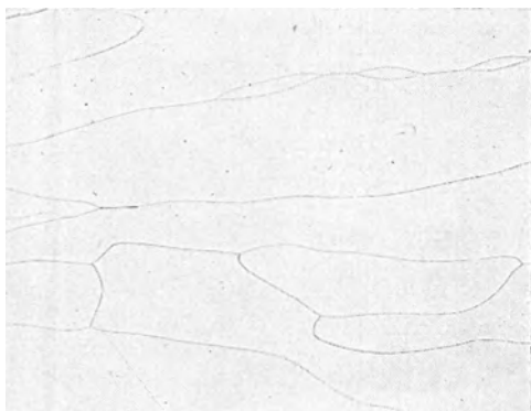
FIG. 7. Microstructure of arc-melted molybdenum, calcium-reduced in the presence of 3% aluminum. Etchant, NH 4 OH-H 2 O 2 . 75X before reduction for publication.
