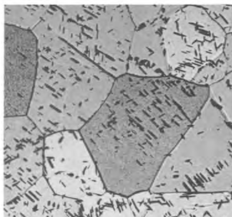
FIG. 10. Cold rolled and annealed structure of electrolytic titanium, 90% reduction, annealed at 800°C, 30 min, air-cooled.
