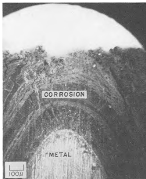
FIG. 4. Positive plate corrosion photographed under dark-field illumination through cover glass and immersion oil. Section was ground on number 600 gritcloth but not polished. Direction of grinding is indicated by metal smear across dark corrosion product. Such smears and surface dirt can be removed with Scotch tape. 100X before reduction for publication.
