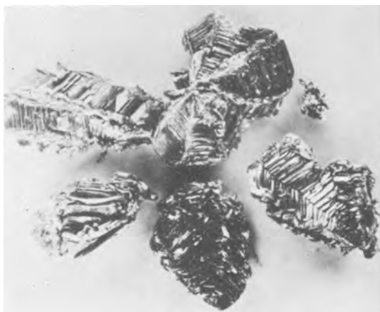
FIG. 7. Typical zirconium metal dendritic crystals
