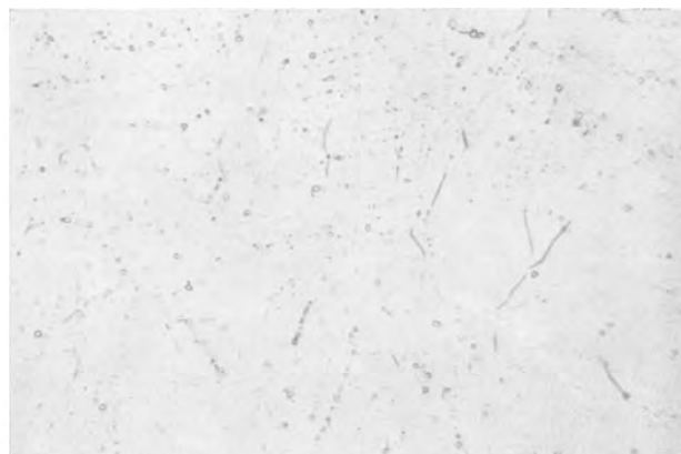
FIG. 12. Zirconium-2.5 wt % tin alloy vacuum annealed at 800°C for 1 hr. Aqua regia-HF etch. 500× before reduction for publication.
