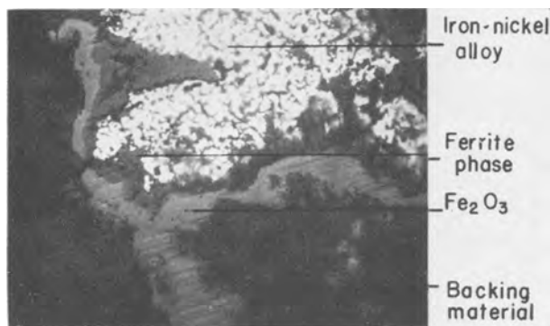
FIG. 3. Oxide film on iron-nickel alloy prepared by sand blasting. Oxidized for 60 min at 700°C. Magnification in vertical direction, 15,000×, in horizontal direction, 1500×, before reduction for publication.
