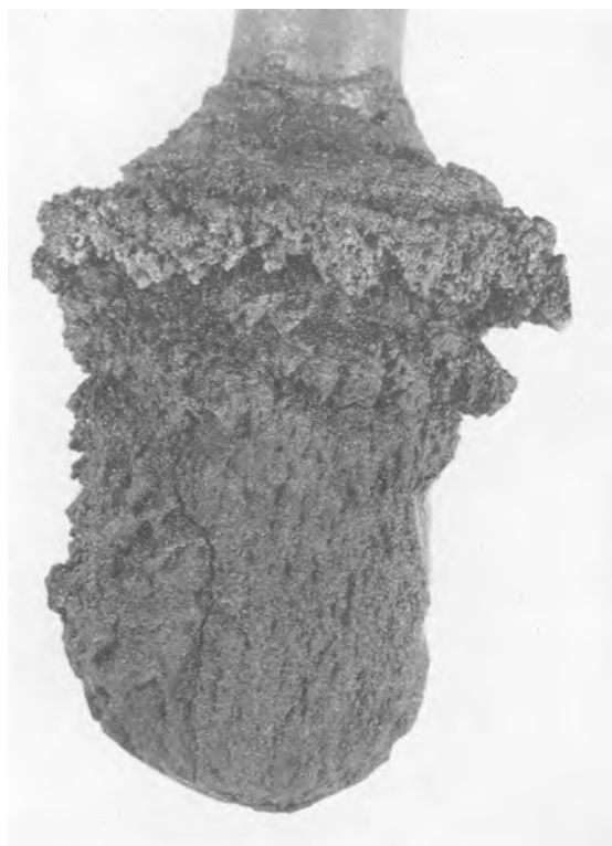
FIG. 2. Typical cathode deposit. Titanium produced by electrolysis of TiO in CaCl 2 .
